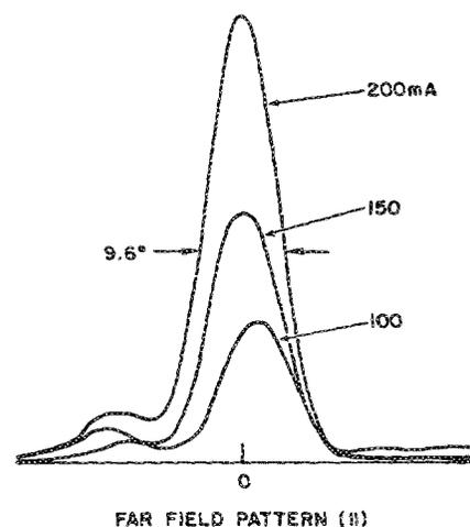
FIG. 4. Far-field pattern parallel to the  $p$ - $n$  junction of a laser diode.
