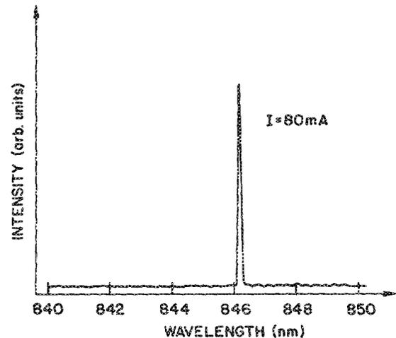
FIG. 3. Lasing spectrum of the same diode shown in Fig. 2. The side mode suppression ratio was 95 to 1 at this pumping current of  $1.6I_{th}$ .
