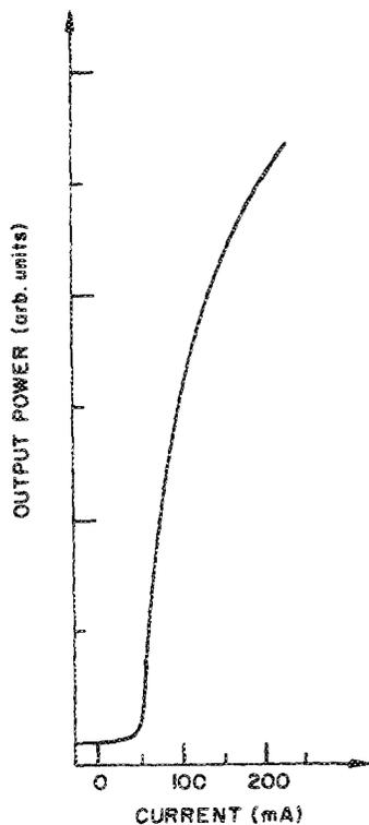
FIG. 2. Power output vs pumping current of a typical laser diode. The threshold current was 50 mA.
